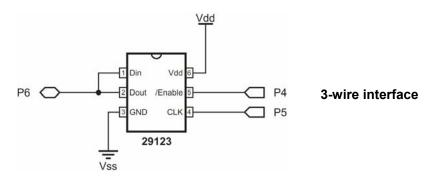
The Din and Dout pins do not have to be tied together; they can also be controlled individually. This makes it possible to share communication lines with other synchronous serial devices that have dedicated input and output lines.
