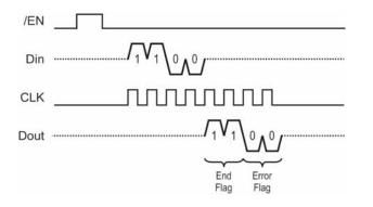
Shifting-in the x and y-axis values is a simple matter of shifting-in 11 bits for the x-axis measurement followed by 11 more bits for the y-axis measurement. After completing the y-axis shift-in, set the /EN pin high again.
