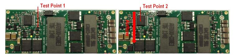
Figure 20 Temperature test point
