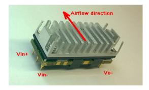
Figure 24 Temperature test point & heat sink mechanical diagram
