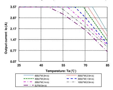
Figure 21 Output power derating, 48V<sub>in</sub>, air flowing across the converter from pin 3 to pin 1
