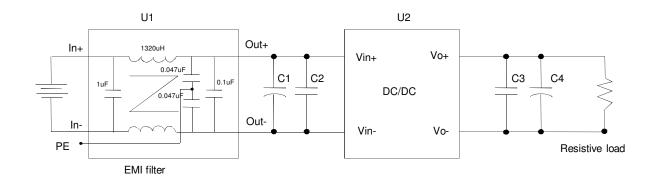
Figure 19 EMC test configuration
