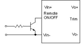
Isolated remote ON/OFF circuit
