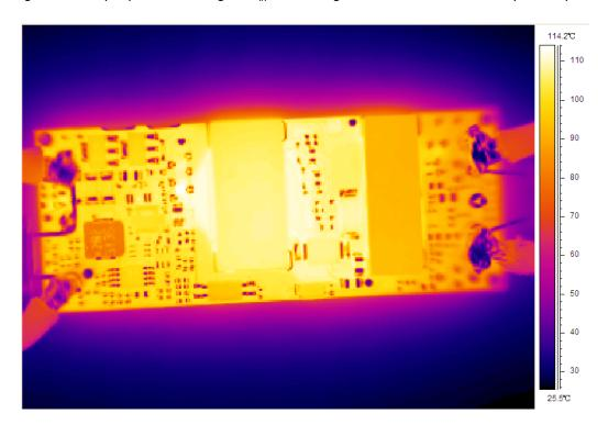
Figure 26 Thermal image,  $36V_{in}$ ,  $28V_{o}$ , full load, room temperature, 200LFM
