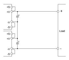
Fig.12-1 Series Operation in High Output Voltage
