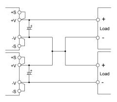
Fig.12-2 ±Output Series Operation
