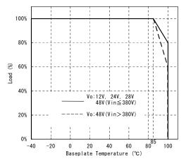
Fig.15-2 Derating curve
