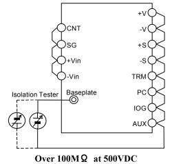
Fig.22-1 Isolation Test
