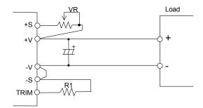
Fig.2-2 Example Connection of External Resistor
