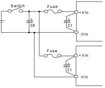
Fig.1-4 Input Filter when Plural Power
