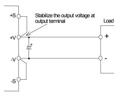
Fig.9-2 Remote Sensing Not in Use
