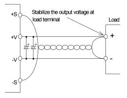
Fig.9-1 Remote Sensing at Use
