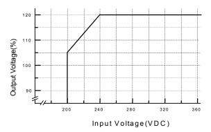
Fig.2-1 Limit of Input Voltage
