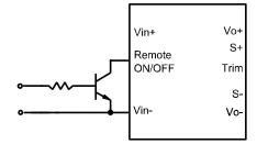
Figure 22 external Remote ON/OFF circuit
