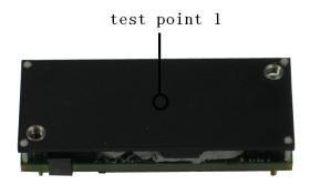
Figure 17 Thermal test points(TOP)
