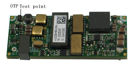
Figure 10 Open Frame Product OTP test poinse
