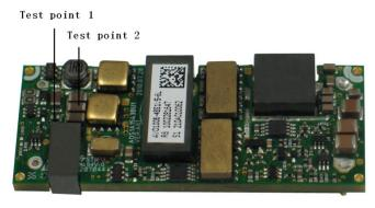
Figure 14 Thermal test points(TOP)
