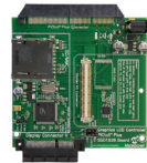
Graphics LCD Controller PICtail™ Plus SSD1926 Board (AC164127-5) (Includes Solomon Systech SSD1926 Controller)
