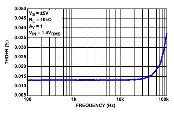
FIGURE 22. TOTAL HARMONIC DISTORTION + NOISE vs FREQUENCY
