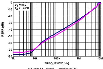
FIGURE 20. PSRR vs FREQUENCY
