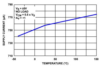
FIGURE 11. SUPPLY CURRENT vs TEMPERATURE
