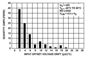
FIGURE 4. INPUT OFFSET VOLTAGE DRIFT (TSOT)
