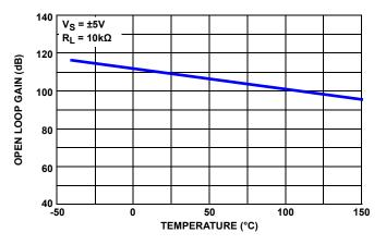
FIGURE 9. OPEN-LOOP GAIN vs TEMPERATURE
