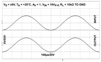
FIGURE 29. OPERATION WITH RAIL-TO-RAIL INPUT AND OUTPUT
