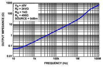
FIGURE 17. CLOSED LOOP OUTPUT IMPEDANCE vs FREQUENCY
