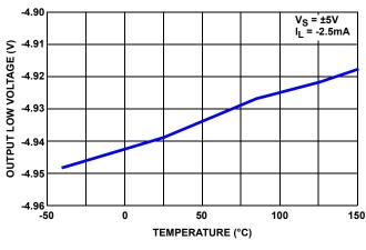
FIGURE 8. OUTPUT LOW VOLTAGE vs TEMPERATURE
