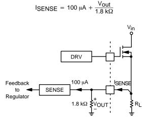
Figure 5. Voltage Regulation Using Sense Feature
