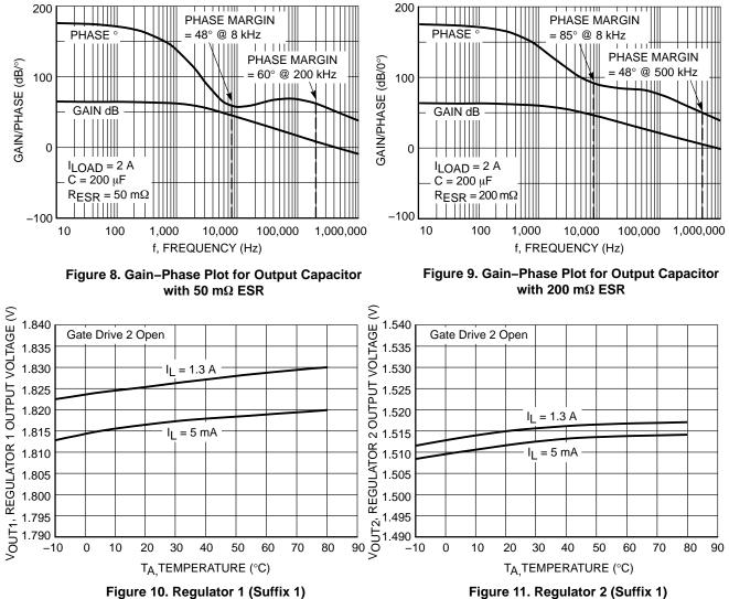
Output Voltage vs. Ambient Temperature
