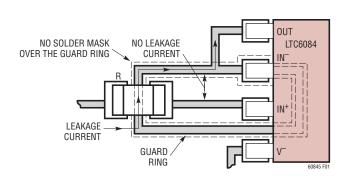
Figure 1. Sample Layout. Unity-Gain Configuration. Using Guard Ring to Shield High Impedance Input from Board Leakage
