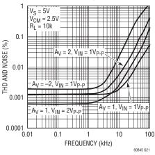
Total Harmonic Distortion and Noise vs Output Voltage
