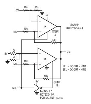
Figure 3. Inverting Amplifier with Muxed Output
