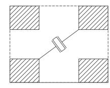
Pad #2 and #4 connected with metal cap
