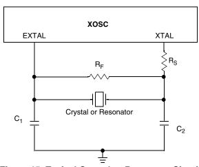
Figure 15. Typical Crystal or Resonator Circuit
