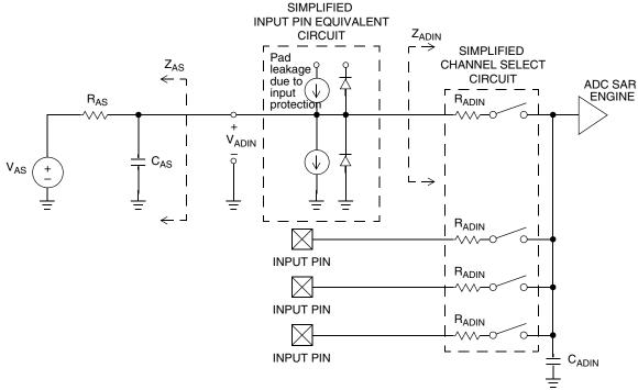
Figure 25. ADC Input Impedance Equivalency Diagram
