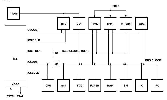
Figure 2. System Clock Distribution Diagram
