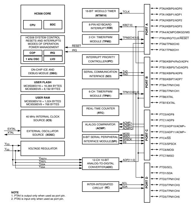
Figure 1. MC9S08SV16 Series Block Diagram
