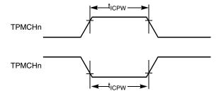
Figure 20. Timer Input Capture Pulse
