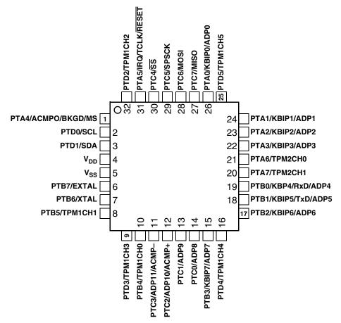
Figure 4. MC9S08SV16 Series 32-Pin LQFP Package
