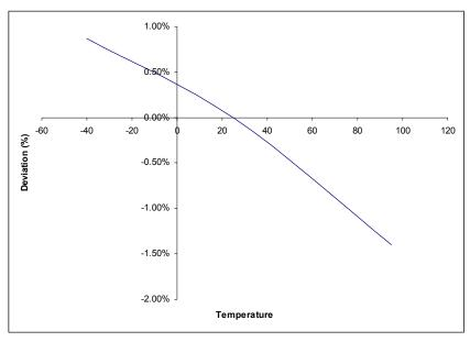
Figure 16. Deviation of DCO Output from Trimmed Frequency (20 MHz, 5.0 V)
