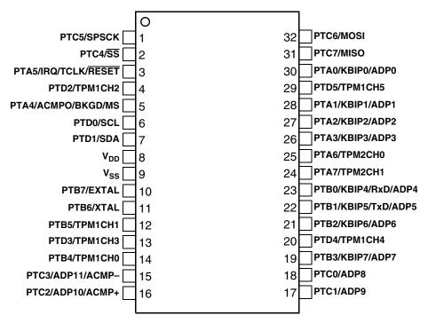
Figure 3. MC9S08SV16 Series 32-Pin SDIP Package
