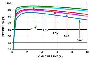
FIGURE 2. EFFICIENCY vs LOAD CURRENT (5VIN)
