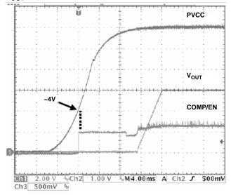
FIGURE 13. POR AND SOFT-START OPERATION
