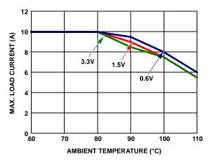
FIGURE 23. DERATING CURVE (5VIN)
