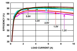
FIGURE 4. EFFICIENCY vs LOAD CURRENT (18VIN)
