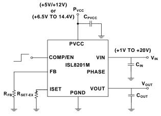
FIGURE 12. WIDE INPUT VOLTAGE APPLICATION SCHEMATIC
