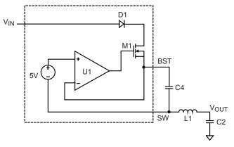
Figure 2—Internal Bootstrap Charging Circuit
