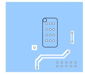
Bottom Layer Figure 7—PCB Layout
