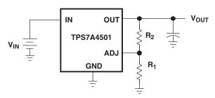
$$\begin{split} &V_{\text{OUT}} = 1.21 \text{ V} \Big( 1 \ + \ \frac{\text{R2}}{\text{R1}} \Big) \ + (I_{\text{ADJ}}) (\text{R2}) \\ &V_{\text{ADJ}} = 1.21 \text{ V} \\ &I_{\text{ADJ}} = 3 \text{ } \mu\text{A} \text{ at } 25^{\circ}\text{C} \\ &\text{Output range} = 1.21 \text{ V to } 20 \text{ V} \end{split}$$
