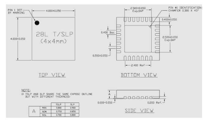
Figure 9-3 QFN-28 Package Dimensions
