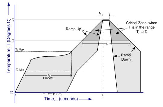
Figure 9-5 FT120 Solder Reflow Profile
