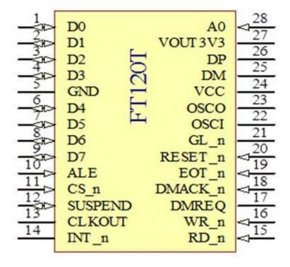
Figure 3-1 TSSOP-28 package schematic symbol
