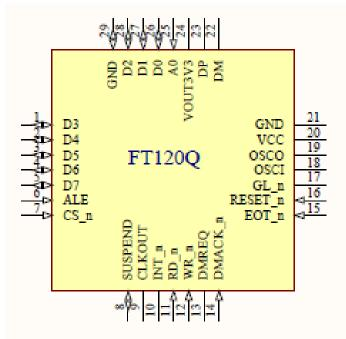
Figure 3-2 QFN-28 package schematic symbol
