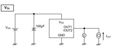
Figure 4. VoL Measurement Circuit
