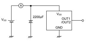
Figure 5. IDD Measurement Circuit
