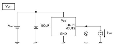
Figure 3. V<sub>OH</sub> Measurement Circuit
