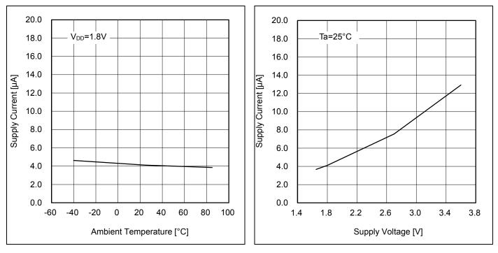
Figure 10. Supply Current vs Ambient Temperature
