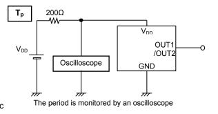
Figure 2.  $T_{\text{p}}$  Measurement Circuit
