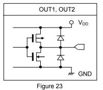
The Hall ICs output pins are configured for CMOS (inverter) output removing the need for external resistance and allow direct connection to the host. Removing the need for external resistors allows for reduction of the current that would otherwise flow to the external resistor during magnetic field detection thereby supporting an overall lower current (micropower) operation.
