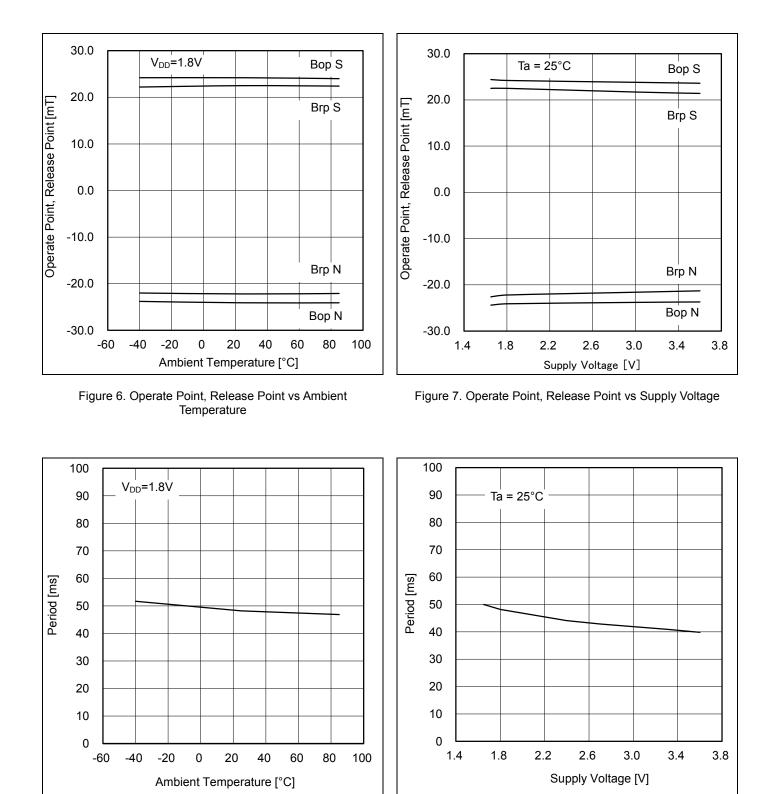
Figure 8. Period vs Ambient Temperature
