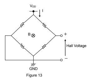
The Hall elements form an equivalent Wheatstone (resistor) bridge circuit. Offset voltage may be generated by a differential in this bridge resistance, or can arise from changes in resistance due to package or bonding stress. A dynamic offset cancellation circuit is employed to cancel this offset voltage.
