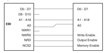
Figure 10 shows how to connect a 512K x 16-bit memory on NCS2.
