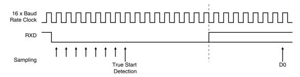
Figure 39. Asynchronous Mode: Character Reception
