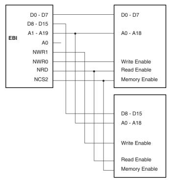
Byte Select Access is used to connect 16-bit devices in a memory page.
