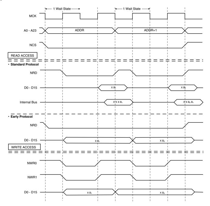
Figure 31. 1 Wait State, 8-bit Bus Width, Byte Transfer
