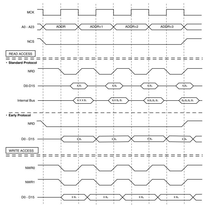
Figure 29. 0 Wait States, 8-bit Bus Width, Word Transfer
