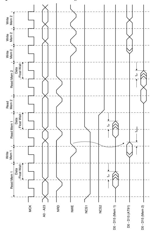
Figure 24. Standard Read Protocol with  $t_{\rm DF}$
