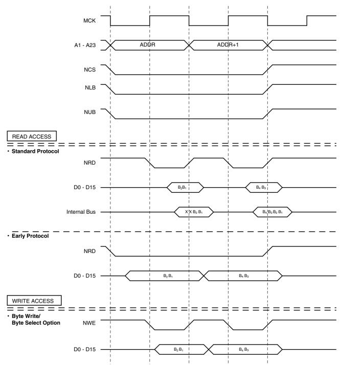
Figure 27. 1 Wait, 16-bit Bus Width, Word Transfer
