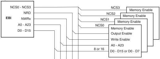
Note: For four external devices, the maximum address space per device is 16M bytes.
