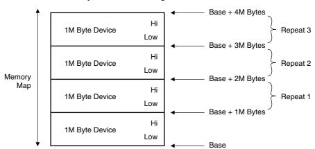
Figure 6. External Memory Smaller than Page Size
