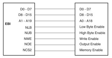
Figure 13 shows how to connect a 16-bit device without byte access (e.g. Flash) on NCS2.
