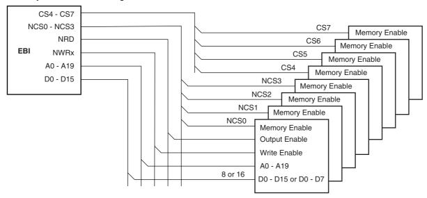
Note: For eight external devices, the maximum address space per device is 1M byte.
