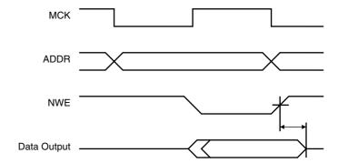
In early read protocol the data can remain valid longer than in standard read protocol due to the additional wait cycle which follows a write access.
