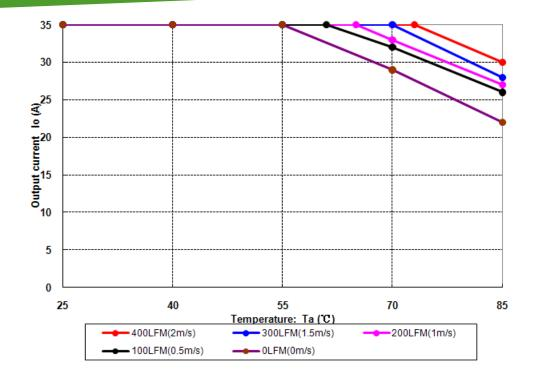
Figure 13 Output power derating, 48Vin, air flowing across the converter from Vin- and Vin+
