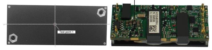
Figure 14 Temperature test point
