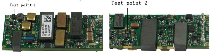
Figure 12 Temperature test point
