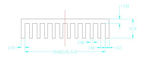
Figure 15 Heatsink (Unit:mm)
