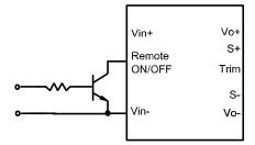
Isolated remote ON/OFF circuit
