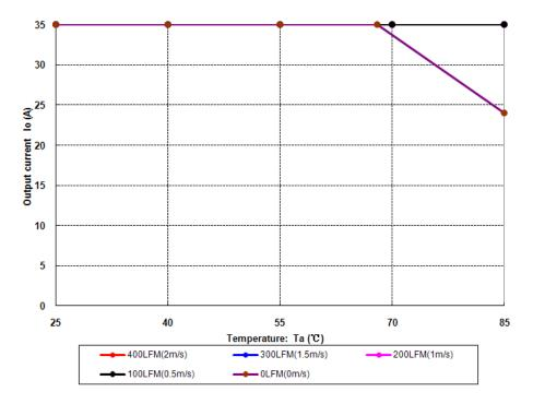
Figure 16 Output power derating, 48Vin, air flowing across the converter from Vin- and Vin+
