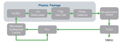
The Vertical Cavity Surface Emitting Laser (VCSEL) replaces the lamp of conventional Rubidium oscillators. The upside of the VCSEL is a reduction in size, weight, and power. The following describes a detailed description of the MAC:
