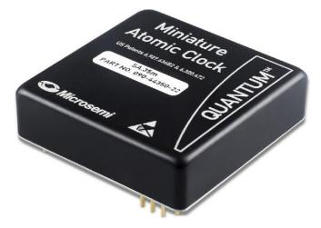
The SA.3Xm is refined for cost effective mass production and can be easily integrated into time, frequency, and synchronization systems. The SA.3Xm requires a single supply voltage and can be mounted directly onto a circuit board as a component of a module used in 20 mm (0.8") wide card slots. The design produces a stable frequency with good short and long term stability, and excellent phase noise performance.
