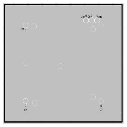
Note: Capacitors in Figure 9 are 6.8 pF, 50 V (Murata p/n GJM1555C1H6R8CB01D, AVX p/n 04025A6R8CAT2A).
