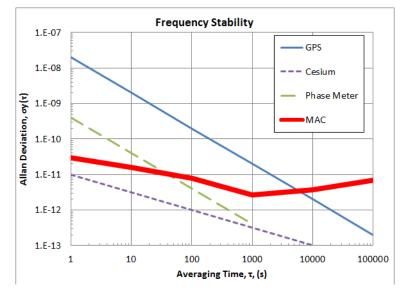
Figure 7 shows typical instability (Allan Deviation) of the MAC (in red), along with the noise floor of the Phase Meter (in green). Also shown are the instabilities of typical reference sources, GPS (in blue) and a high-performance Cesium Beam frequency standard (in purple). When disciplining, the stability of the output of the MAC at any averaging time reflects the noise properties of the dominant (most noisy) source.
