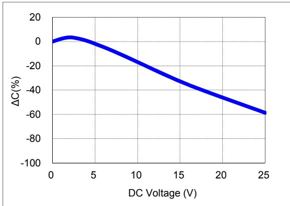
4) Bias TCC characteristics (Agilent 4284A, 1kHz, 1.0Vrms, 12.5Vdc)
