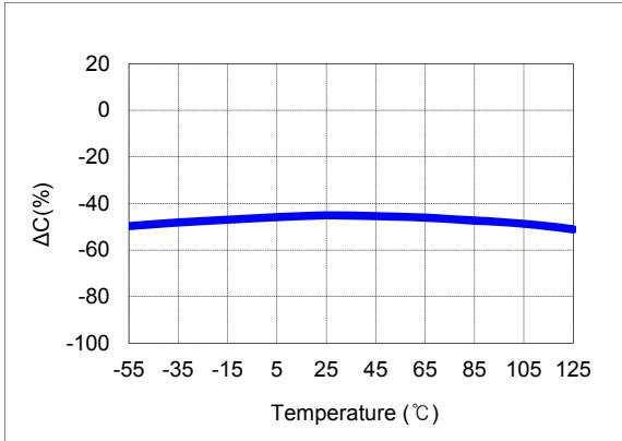
5) AC voltage characteristics (Agilent 4284A, 1kHz)
