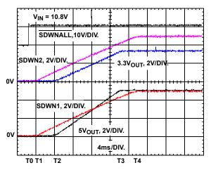
FIGURE 7. SOFT-START ON 3.3V AND 5V OUTPUTS
