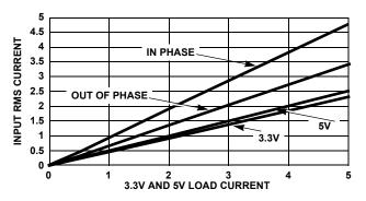
FIGURE 9. INPUT RMS CURRENT vs LOAD
