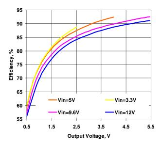
Figure 6. Efficiency vs. Output Voltage, lout=7A
