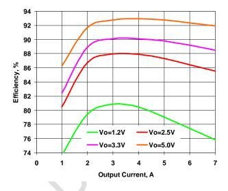
Figure 4. Efficiency vs. Load. Vin=9.6V
