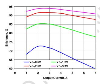
Figure 3. Efficiency vs. Load. Vin=5V
