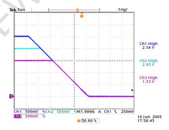
Figure 9. Tracking Turn-Off Vin=12V, Ch1 - V1, Ch2 - V2, Ch3 - V3
