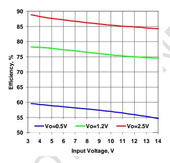
Figure 7. Efficiency vs. Input Voltage. lout=7A
