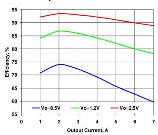
Figure 2. Efficiency vs. Load. Vin=3.3V
