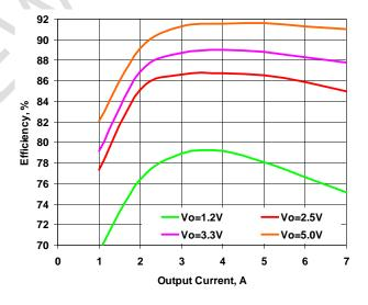
Figure 5. Efficiency vs. Load. Vin=12V
