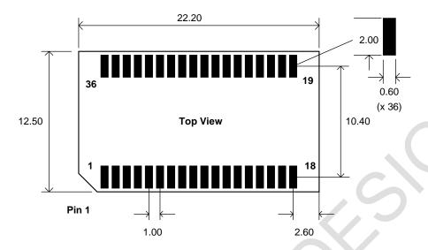
Figure 24. Recommended PCB Pad Sizes
