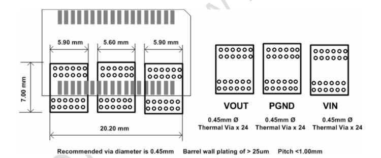
Figure 25. Recommended PCB Layout for Multilayer PCBs
