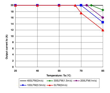
Figure 12 Derating curve
