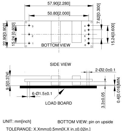
OLERANCE: X.Xmm $\pm 0.5$ mm[X.X in. $\pm 0.02$ in.] X.XXmm $\pm 0.25$ mm[X.XX in. $\pm 0.01$ in.]
