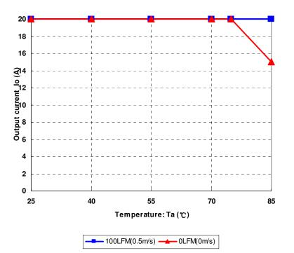
Figure 16 Derating curve
