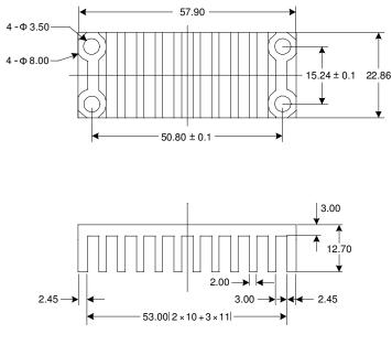
Figure 15 Heatsink (Unit:mm)
