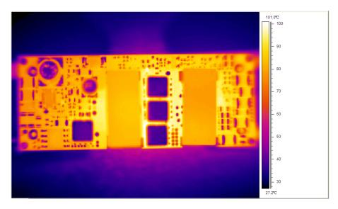
Figure 17 Thermal image, 48V<sub>in</sub>, 5V<sub>o</sub>, full load, room temperature, 100LFM (air flowing from pin 1 to pin 3)
