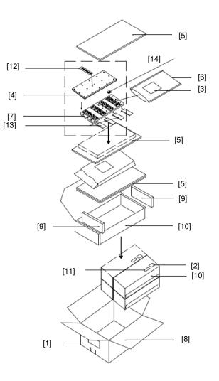
Figure 24 Package disassembly
