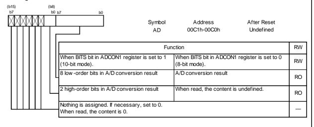
Figure 18.3 Registers ADCON1, ADCON2, and AD
