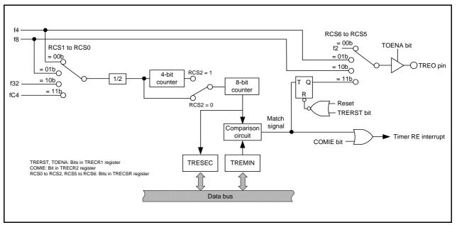
Figure 14.123 Block Diagram of Output Compare Mode
