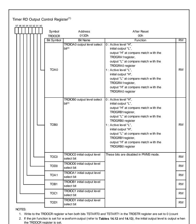
Figure 14.101 TRDOCR Register in PWM3 Mode
