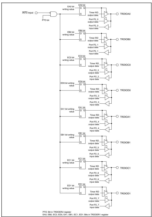
**Figure 14.31 Pulse Output Forced Cutoff**
