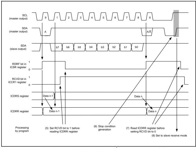
Operating Timing in Master Receive Mode (I<sup>2</sup>C bus Interface Mode) (2) **Figure 16.36**
