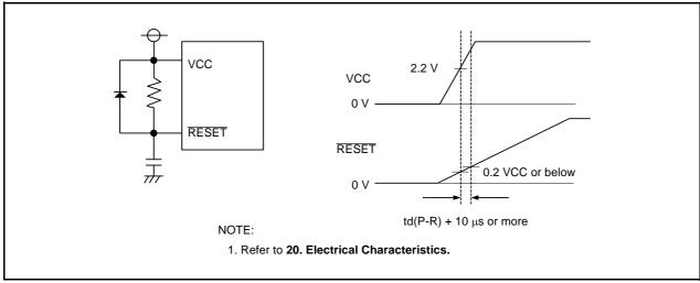
Figure 5.5 Example of Hardware Reset Circuit and Operation
