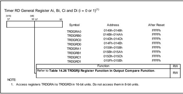
Figure 14.58 Registers TRDGRAi, TRDGRBi, TRDGRCi, and TRDGRDi in Output Compare Function
