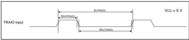
Figure 20.9 TRAIO Input Timing Diagram when Vcc = 5 V
