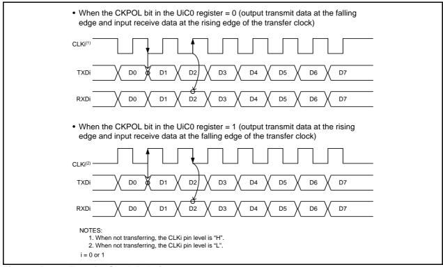
Figure 15.8 Transfer Clock Polarity
