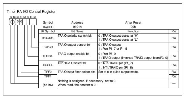
Figure 14.6 **TRAIOC Register in Pulse Output Mode**
