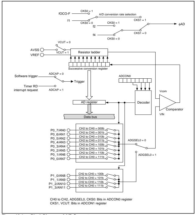
Figure 18.1 **Block Diagram of A/D Converter**
