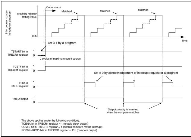
Figure 14.129 Operating Example in Output Compare Mode
