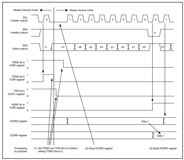
Operating Timing in Master Receive Mode (I<sup>2</sup>C bus Interface Mode) (1) **Figure 16.35**
