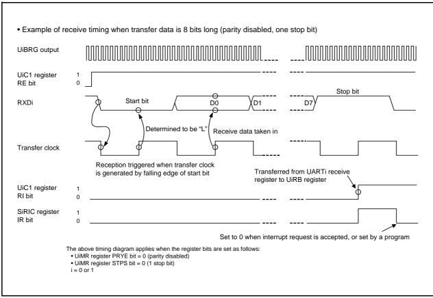
**Figure 15.11 Receive Timing Example in UART Mode**
