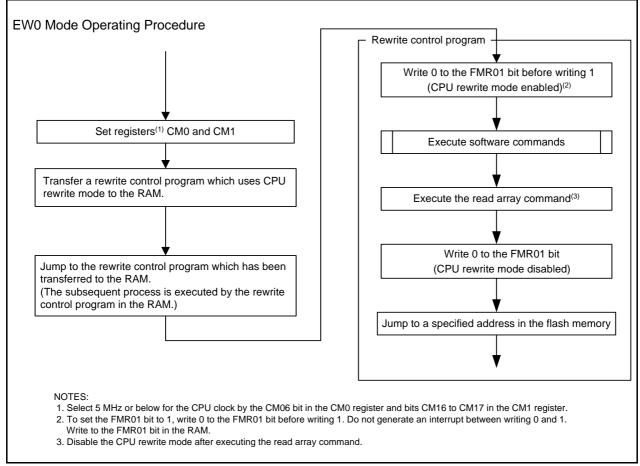
Figure 19.9 How to Set and Exit EW0 Mode
