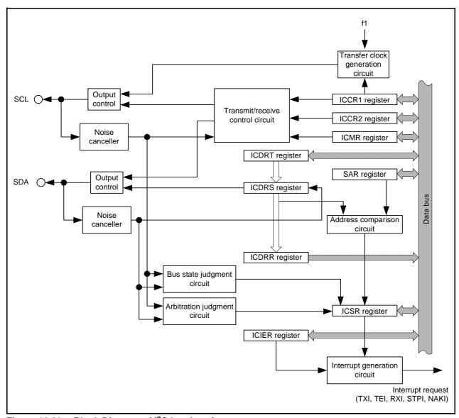
Figure 16.22 Block Diagram of I<sup>2</sup>C bus interface
