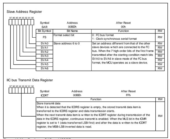
Figure 16.29 Registers SAR and ICDRT
