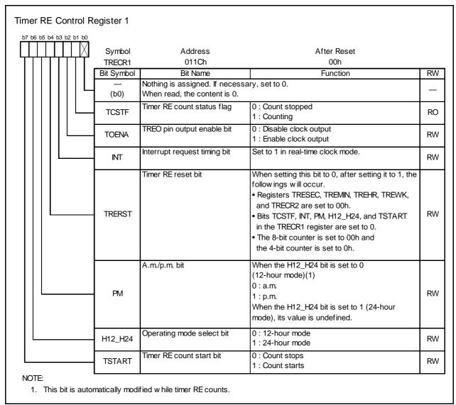
Figure 14.118 TRECR1 Register in Real-Time Clock Mode
