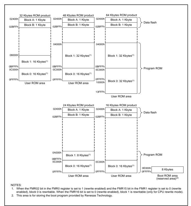
Figure 19.2 Flash Memory Block Diagram for R8C/25 Group
