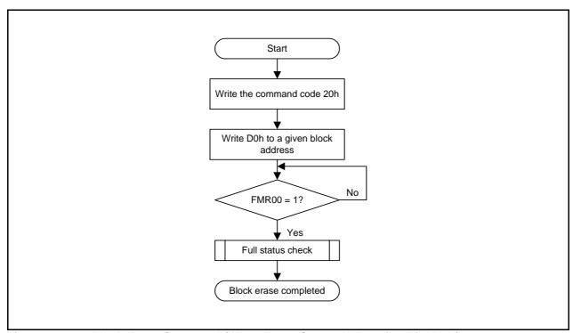
Figure 19.14 Block Erase Command (When Erase-Suspend Function Disabled)
