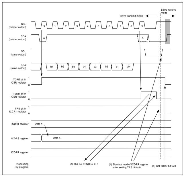
Operating Timing in Slave Transmit Mode (I<sup>2</sup>C bus Interface Mode) (2) **Figure 16.38**
