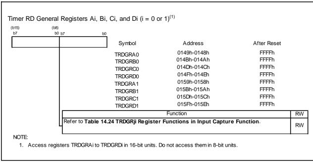
Figure 14.43 Registers TRDGRAi, TRDGRBi, TRDGRCi, and TRDGRDi in Input Capture Function
