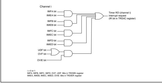
Figure 12.19 Block Diagram of Timer RD Interrupt
