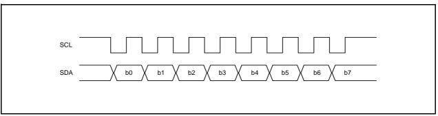
Figure 16.41 Transfer Format of Clock Synchronous Serial Format
