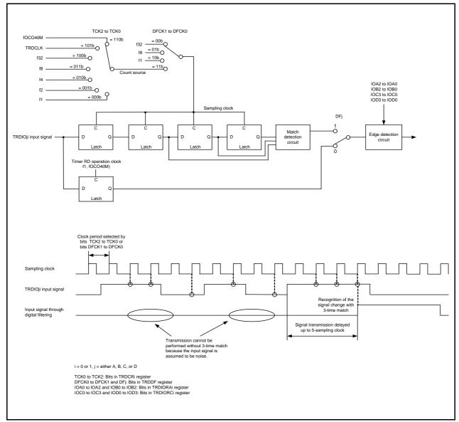
Figure 14.45 Block Diagram of Digital Filter
