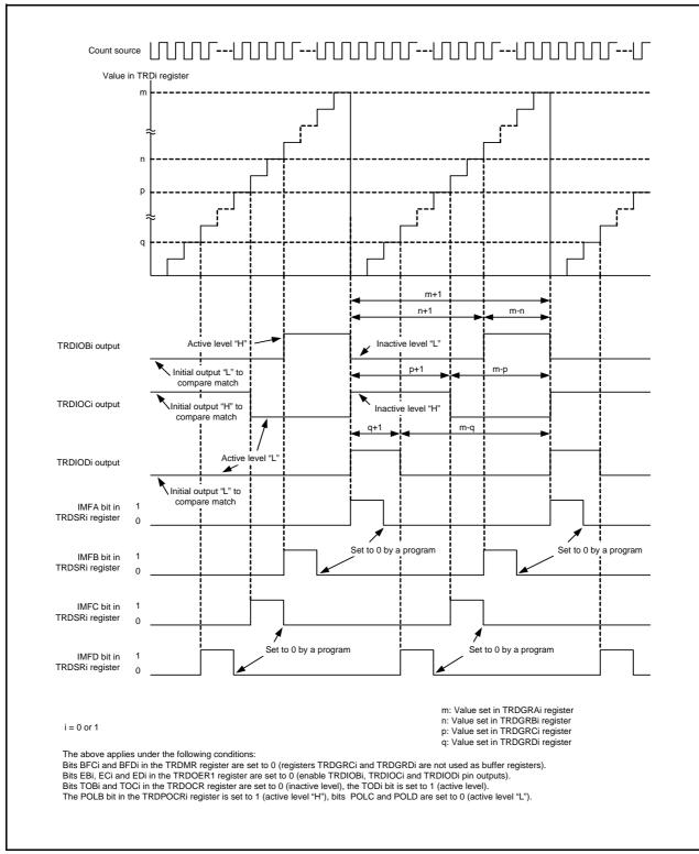
Figure 14.73 Operating Example of PWM Mode
