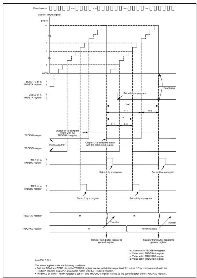
Figure 14.107 Operating Example of PWM3 Mode
