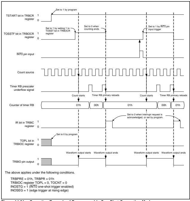
Figure 14.21 Operating Example of Programmable One-Shot Generation Mode
