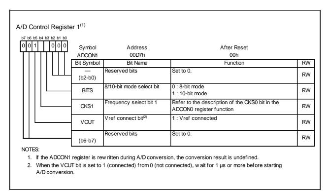
Figure 18.5 **ADCON1 Register in One-Shot Mode**
