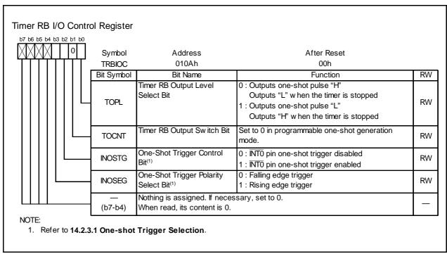
**Figure 14.20 TRBIOC Register in Programmable One-Shot Generation Mode**
