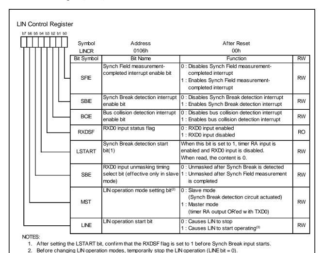
Inputs to timer RA and UART0 are prohibited immediately after this bit is set to 1. (Refer to Figure 17.5 Example of Header Field Transmission Flowchart (1) and Figure 17.9 Example of Header Field Reception Flowchart
