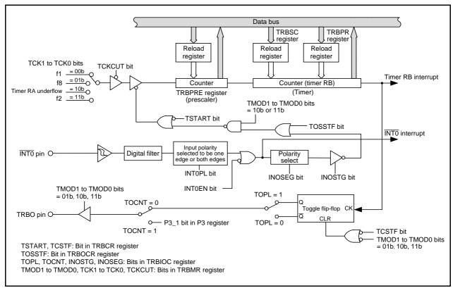
Figure 14.12 Block Diagram of Timer RB
