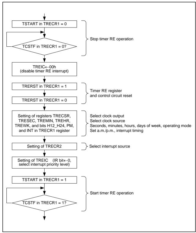
Figure 14.130 Setting Example in Real-Time Clock Mode
