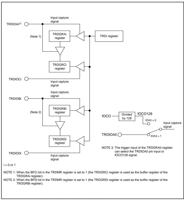
Figure 14.32 Block Diagram of Input Capture Function
