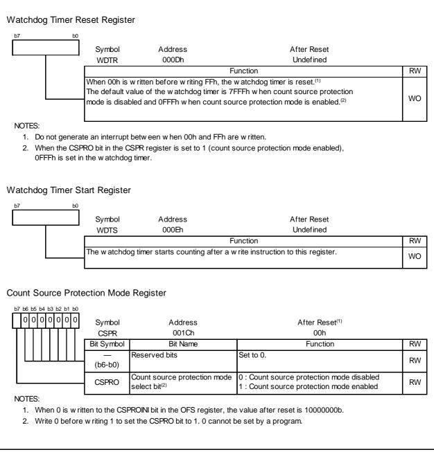
Figure 13.3 Registers WDTR, WDTS, and CSPR
