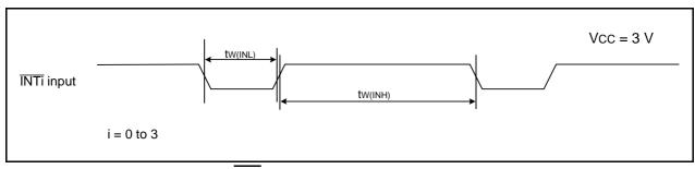
Figure 20.15 External Interrupt INTi Input Timing Diagram when Vcc = 3 V
