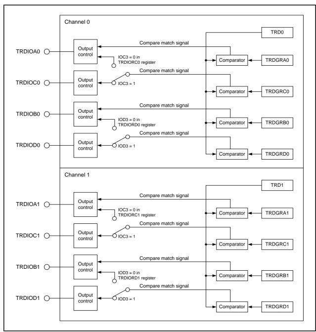
Figure 14.46 Block Diagram of Output Compare Function
