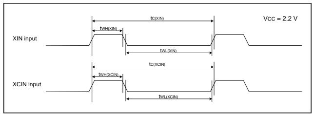
Figure 20.16 XIN Input and XCIN Input Timing Diagram when Vcc = 2.2 V
