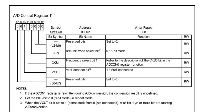
Figure 18.7 **ADCON1 Register in Repeat Mode**
