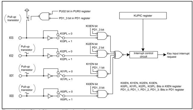
Figure 12.16 Block Diagram of Key Input Interrupt
