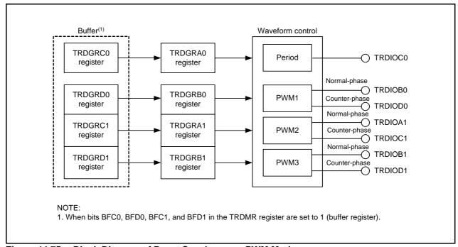
Figure 14.75 Block Diagram of Reset Synchronous PWM Mode
