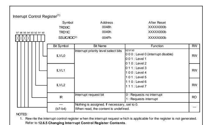
Figure 12.4 Registers TRD0IC, TRD1IC, SSUIC, and IICIC
