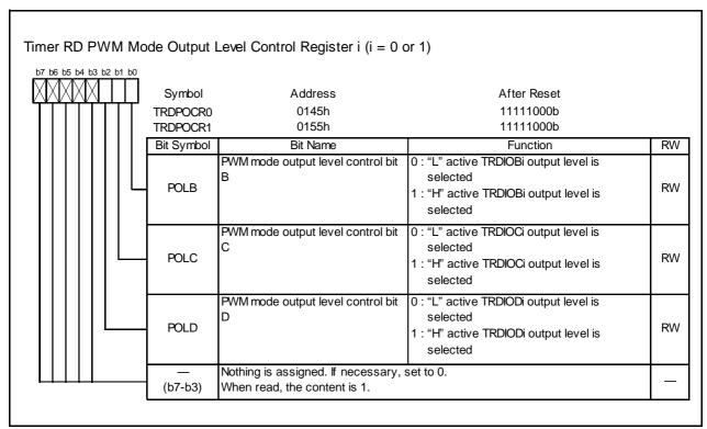
**Figure 14.70** Registers TRDPOCR0 to TRDPOCR1 in PWM Mode
