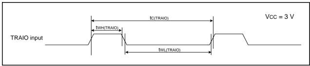
Figure 20.13 TRAIO Input Timing Diagram when Vcc = 3 V
