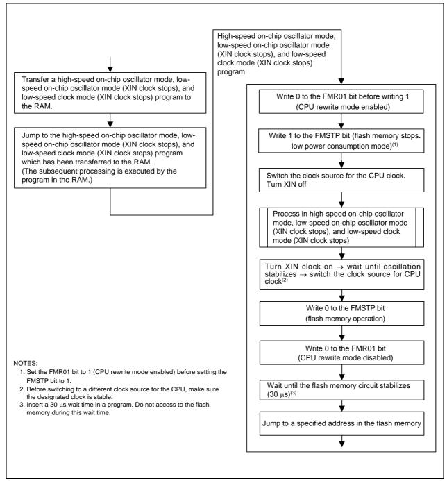
**Figure 19.11** Process to Reduce Power Consumption in High-Speed On-Chip Oscillator Mode, Low-Speed On-Chip Oscillator Mode (XIN Clock Stops) and Low-Speed Clock Mode (XIN Clock Stops)
