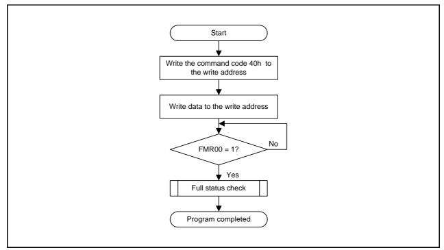
Figure 19.12 Program Command (When Suspend Function Disabled)
