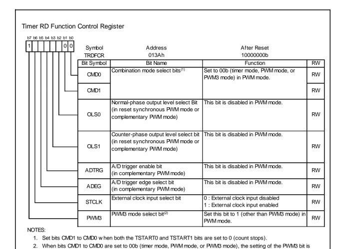
**Figure 14.65 TRDFCR Register in PWM Mode**
