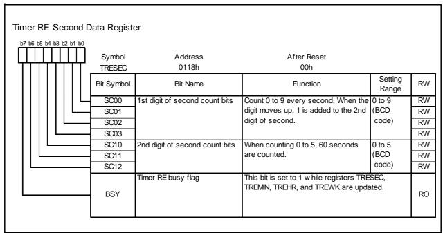
Figure 14.114 TRESEC Register in Real-Time Clock Mode
