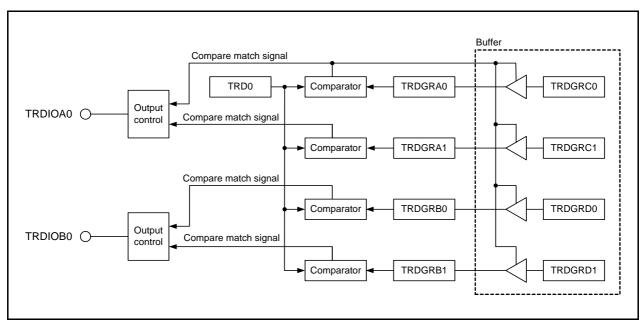
Figure 14.97 Block Diagram of PWM3 Mode
