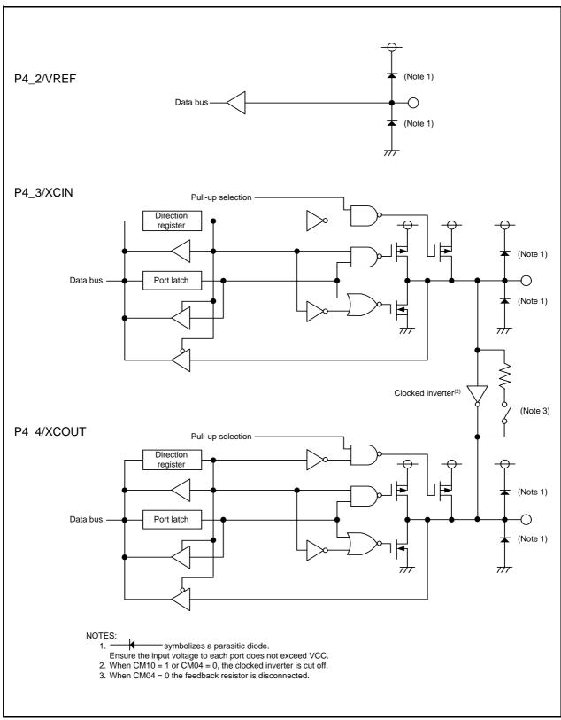
Configuration of Programmable I/O Ports (4) Figure 7.4
