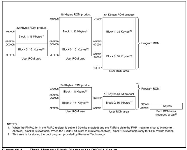
Figure 19.1 Flash Memory Block Diagram for R8C/24 Group
