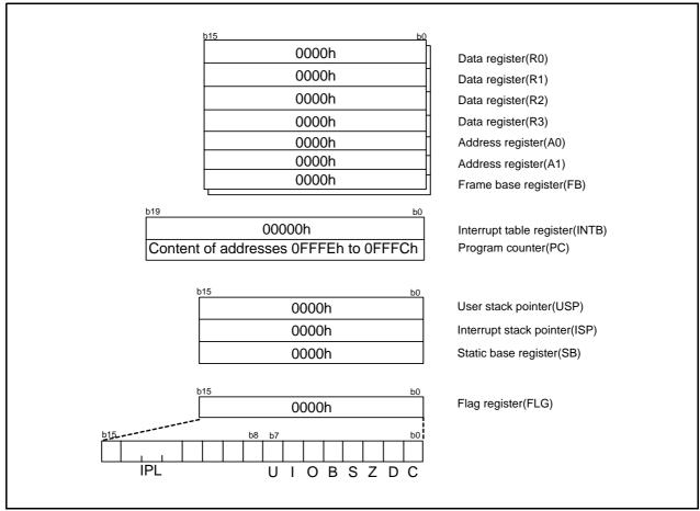
Figure 5.2 **CPU Register Status after Reset**
