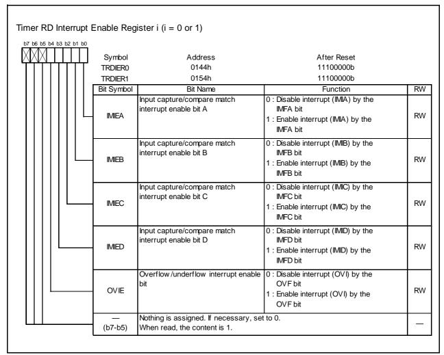
Figure 14.104 Registers TRDIER0 to TRDIER1 in PWM3 Mode
