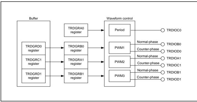
Figure 14.85 Block Diagram of Complementary PWM Mode
