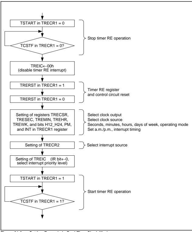
Figure 21.8 **Setting Example in Real-Time Clock Mode**
