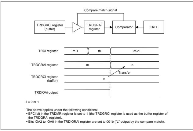
Figure 14.29 Buffer Operation in Output Compare Function
