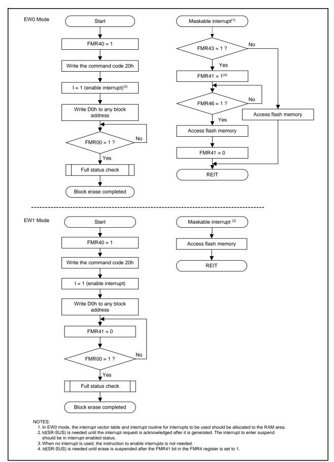
Figure 19.15 Block Erase Command (When Erase-Suspend Function Enabled)
