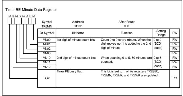
Figure 14.115 TREMIN Register in Real-Time Clock Mode
