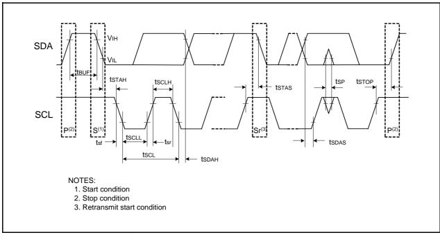
Figure 20.7 I/O Timing of I<sup>2</sup>C bus Interface
