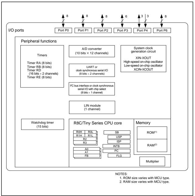
Figure 1.1 Block Diagram
