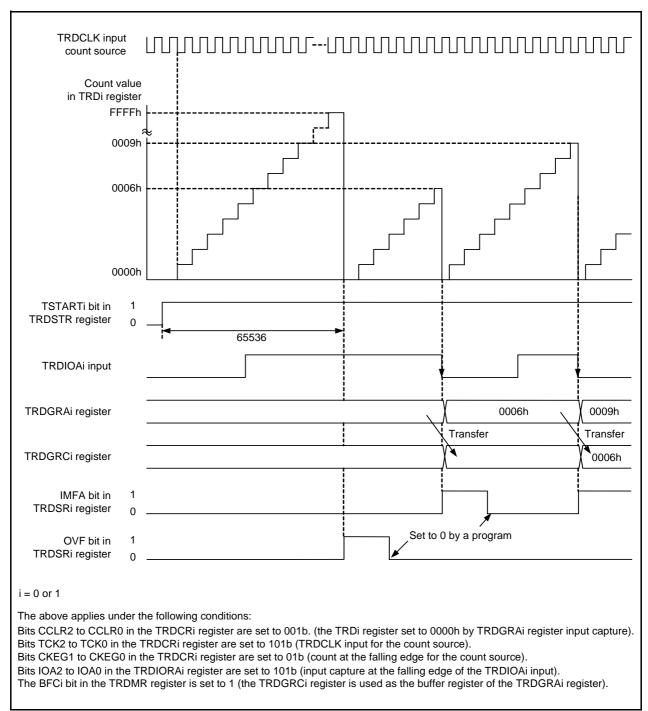
Figure 14.44 Operating Example of Input Capture Function
