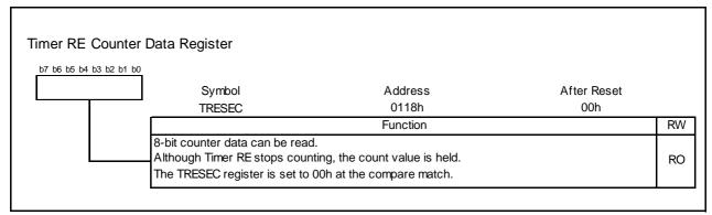
Figure 14.124 TRESEC Register in Output Compare Mode
