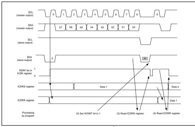
Figure 16.40 Operating Timing in Slave Receive Mode (I<sup>2</sup>C bus Interface Mode) (2)
