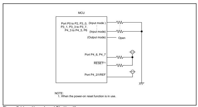
Figure 7.14 Unassigned Pin Handling
