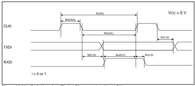
Figure 20.10 Serial Interface Timing Diagram when Vcc = 5 V
