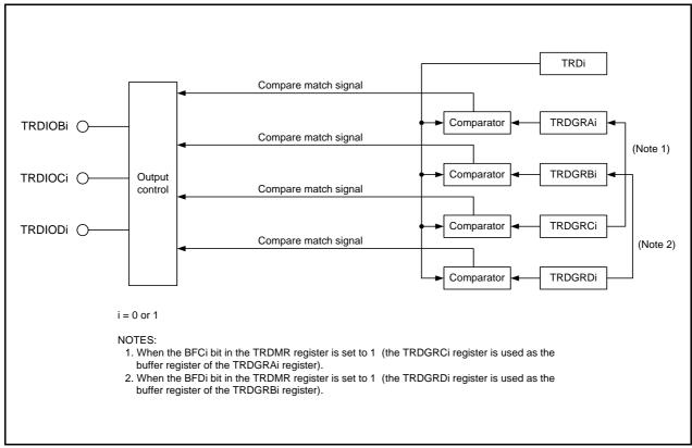
Figure 14.62 Block Diagram of PWM Mode
