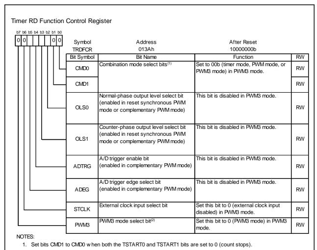
**Figure 14.99 TRDFCR Register in PWM3 Mode**
