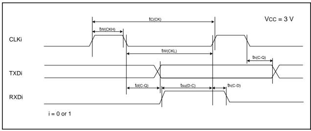
Figure 20.14 Serial Interface Timing Diagram when Vcc = 3 V
