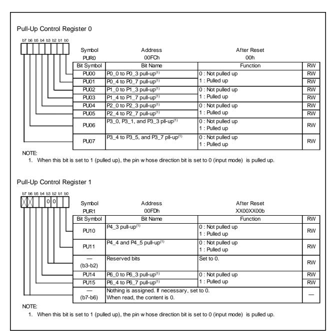
Figure 7.11 Registers PUR0 and PUR1
