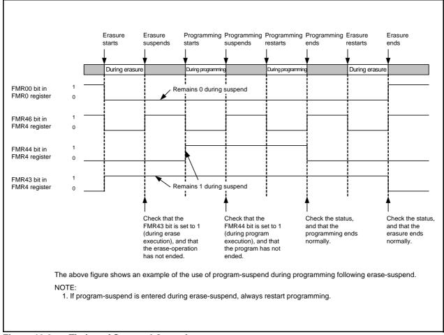
Figure 19.8 Timing of Suspend Operation
