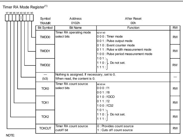
1. When both the TSTART and TCSTF bits in the TRACR register are set to 0 (count stops), rew rite this register.
