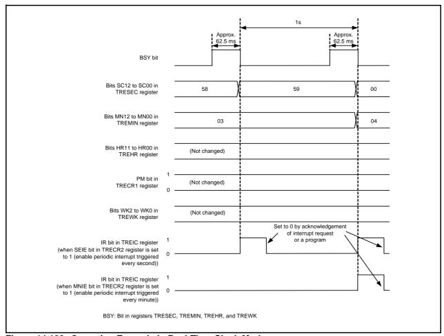
Figure 14.122 Operating Example in Real-Time Clock Mode
