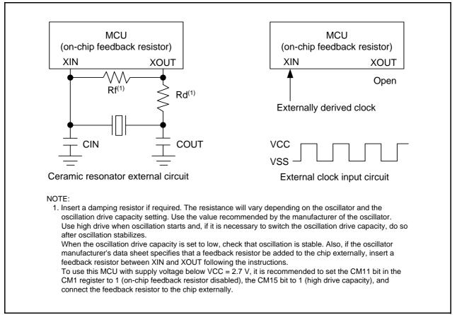
Figure 10.10 Examples of XIN Clock Connection Circuit
