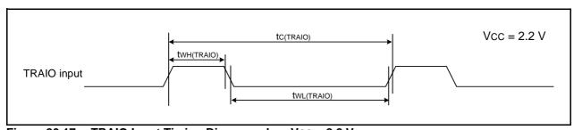
Figure 20.17 TRAIO Input Timing Diagram when Vcc = 2.2 V
