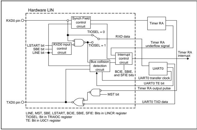
Figure 17.1 Block Diagram of Hardware LIN
