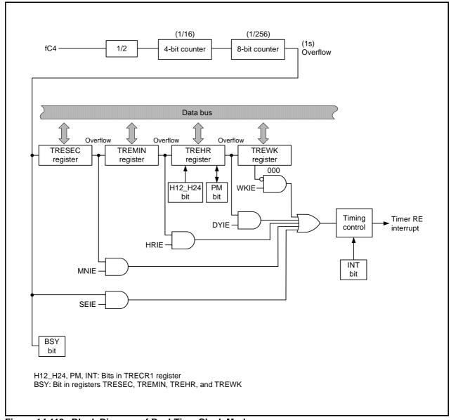
Figure 14.113 Block Diagram of Real-Time Clock Mode
