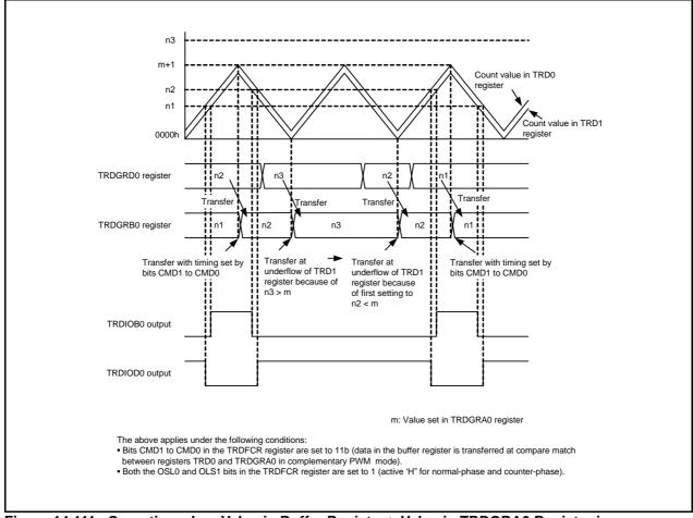
Figure 14.111 Operation when Value in Buffer Register ≥ Value in TRDGRA0 Register in Complementary PWM Mode
