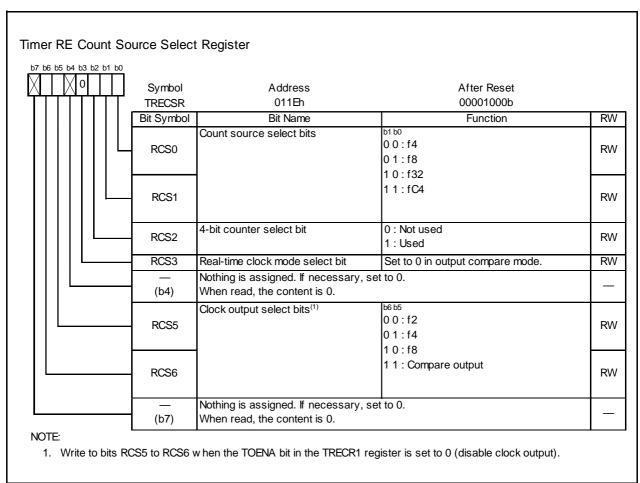
Figure 14.128 TRECSR Register in Output Compare Mode
