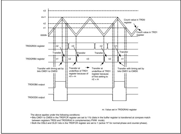
Figure 21.6 Operation when Value in Buffer Register ≥ Value in TRDGRA0 Register in Complementary PWM Mode
