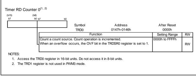
Figure 14.105 TRD0 Register in PWM3 Mode
