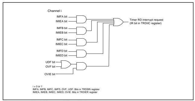
Figure 14.108 Block Diagram of Timer RD Interrupt
