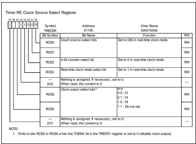
Figure 14.121 TRECSR Register in Real-Time Clock Mode
