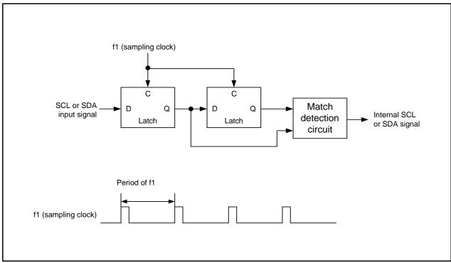
Figure 16.44 Block Diagram of Noise Canceller
