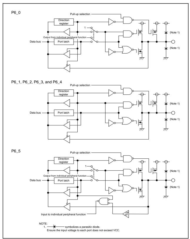
Configuration of Programmable I/O Ports (6) Figure 7.6
