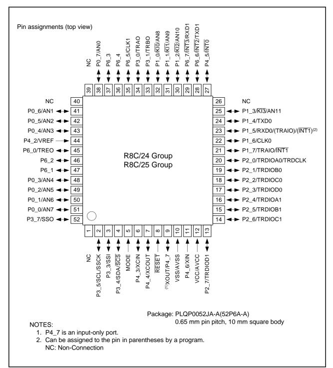
Figure 1.4 PLQP0052JA-A Package Pin Assignments (Top View)
