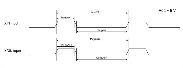
Figure 20.8 XIN Input and XCIN Input Timing Diagram when Vcc = 5 V
