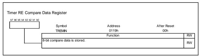
Figure 14.125 TREMIN Register in Output Compare Mode
