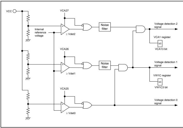
**Block Diagram of Voltage Detection Circuit** Figure 6.1
