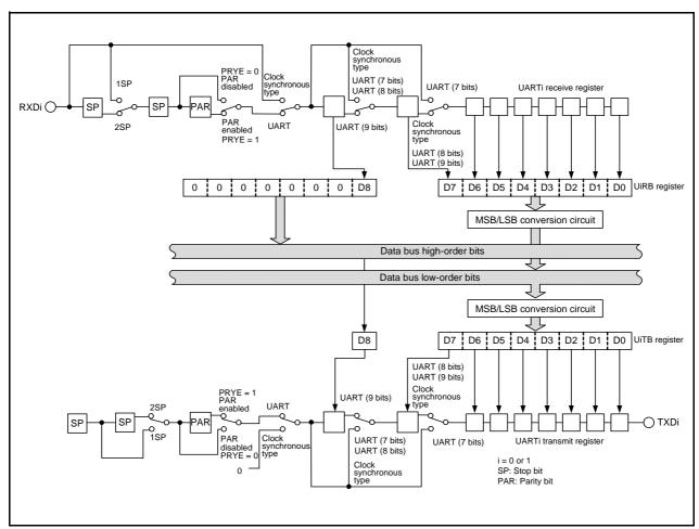
Figure 15.2 UARTi Transmit/Receive Unit
