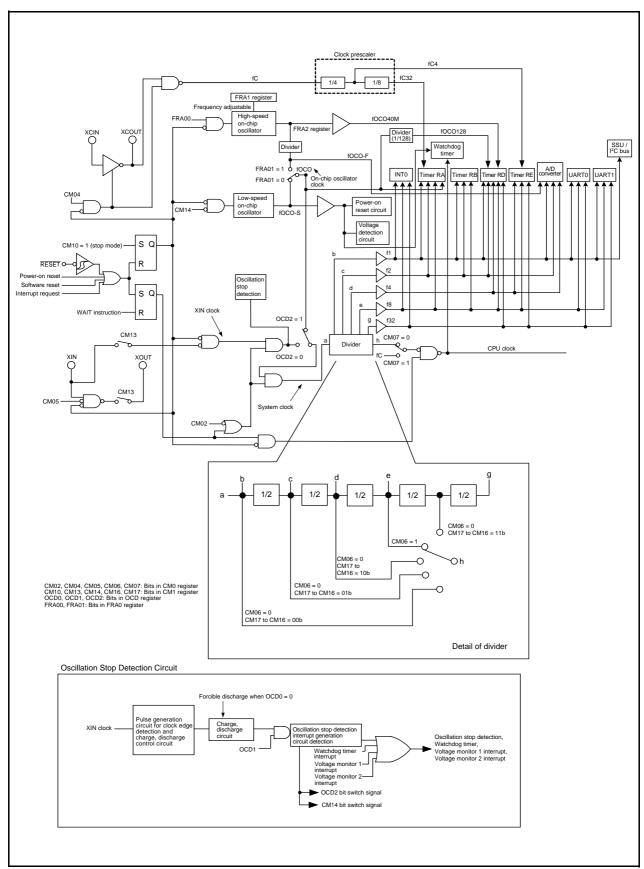
Figure 10.1 **Clock Generation Circuit**
