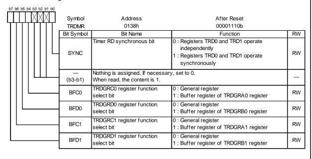
Figure 14.63 Registers TRDSTR and TRDMR in PWM Mode
