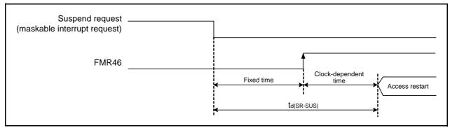
Figure 20.2 Time delay until Suspend
