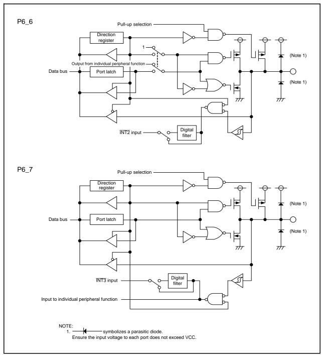
Figure 7.7 Configuration of Programmable I/O Ports (7)
