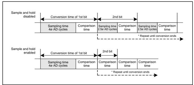
Figure 18.8 Timing Diagram of A/D Conversion
