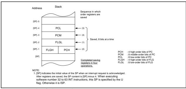
Figure 12.9 Register Saving Operation
