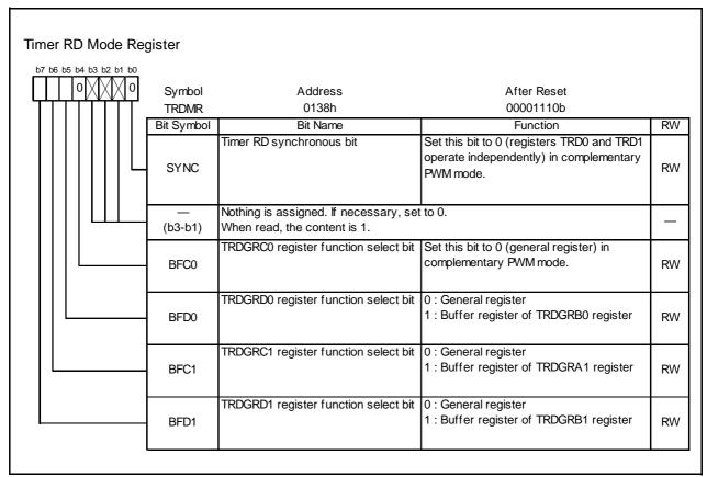
**Figure 14.87 TRDMR Register in Complementary PWM Mode**
