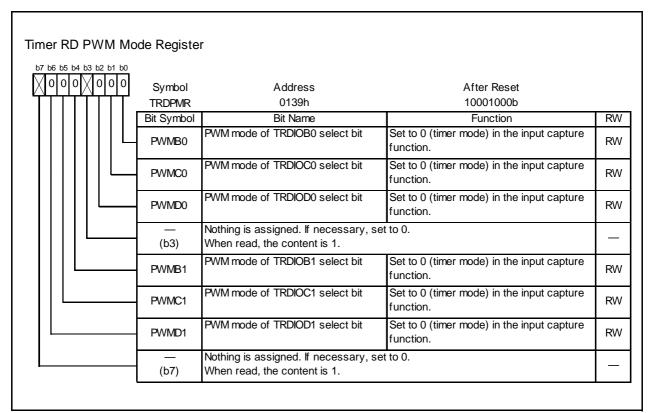
**Figure 14.34 TRDPMR Register in Input Capture Function**
