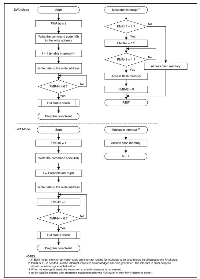
**Figure 19.13 Program Command (When Suspend Function Enabled)**
