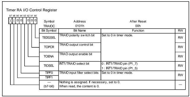
Figure 14.4 TRAIOC Register in Timer Mode
