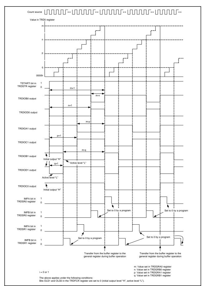
Figure 14.84 Operating Example of Reset Synchronous PWM Mode
