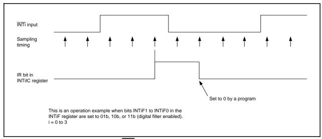
Figure 12.15 Operating Example of INTi Input Filter
