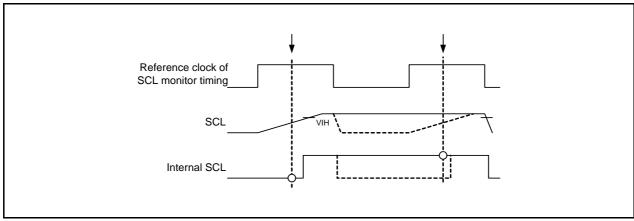
Figure 16.45 Timing of Bit Synchronization Circuit
