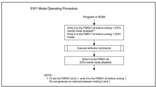
Figure 19.10 How to Set and Exit EW1 Mode
