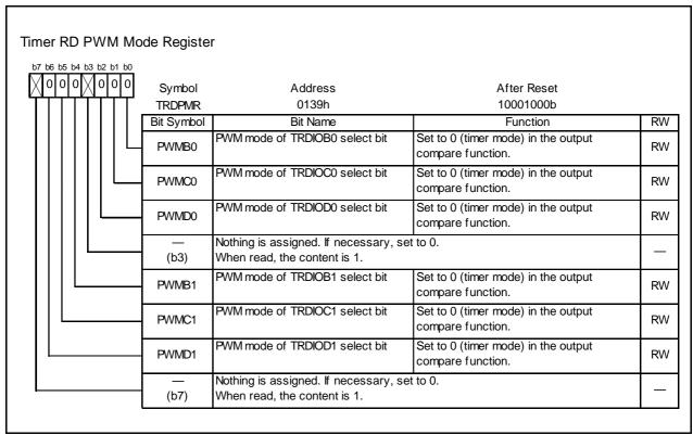
**Figure 14.48 TRDPMR Register in Output Compare Function**
