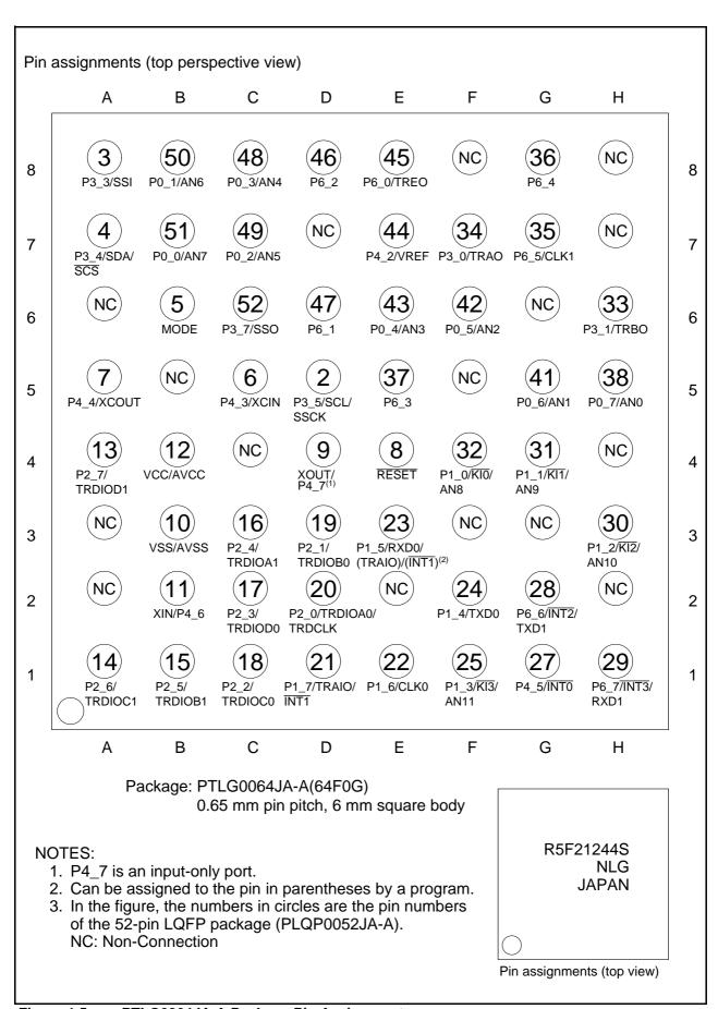
Figure 1.5 PTLG0064JA-A Package Pin Assignments
