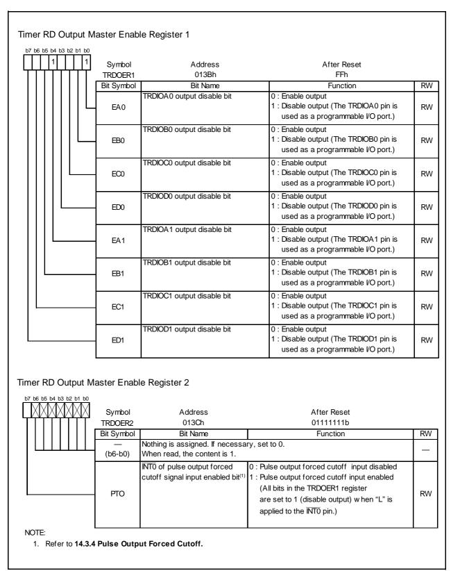
**Figure 14.66** Registers TRDOER1 to TRDOER2 in PWM Mode
