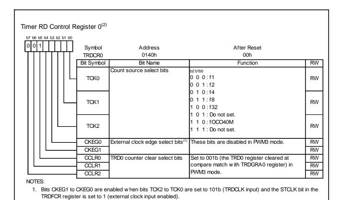
2. The TRDCR1 register is not used in PWM3 mode.
