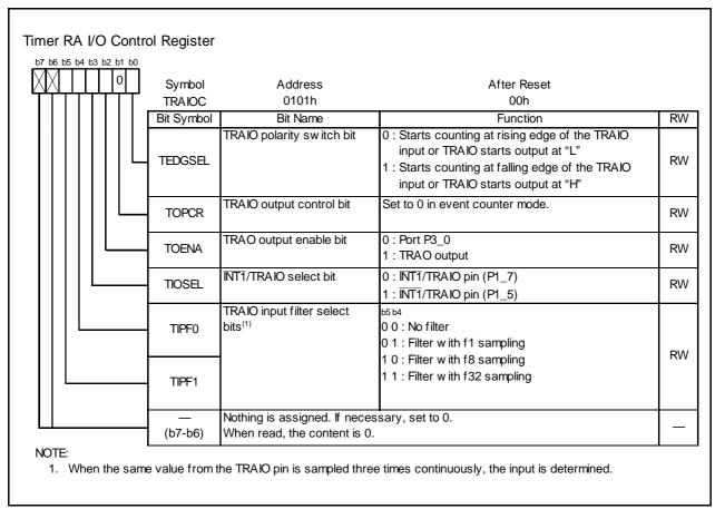
Figure 14.7 TRAIOC Register in Event Counter Mode
