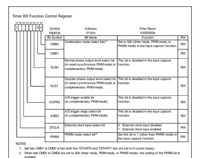
Figure 14.35 TRDFCR Register in Input Capture Function
