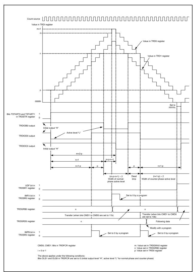
Figure 14.96 Operating Example of Complementary PWM Mode
