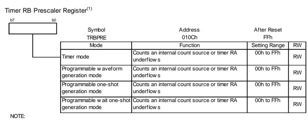
1. When the TSTOP bit in the TRBCR register is set to 1, the TRBPRE register is set to FFh.
