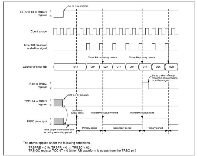
Figure 14.19 Operating Example of Timer RB in Programmable Waveform Generation Mode
