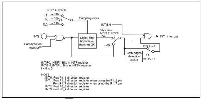
Figure 12.14 Configuration of INTi Input Filter
