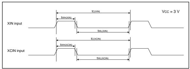
Figure 20.12 XIN Input and XCIN Input Timing Diagram when Vcc = 3 V
