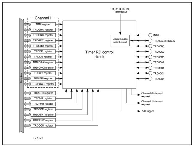
Figure 14.26 Block Diagram of Timer RD
