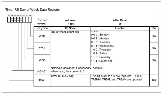
Figure 14.117 TREWK Register in Real-Time Clock Mode
