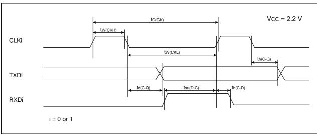
Figure 20.18 Serial Interface Timing Diagram when Vcc = 2.2 V
