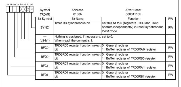
Figure 14.76 Registers TRDSTR and TRDMR in Reset Synchronous PWM Mode
