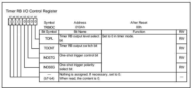
Figure 14.16 TRBIOC Register in Timer Mode
