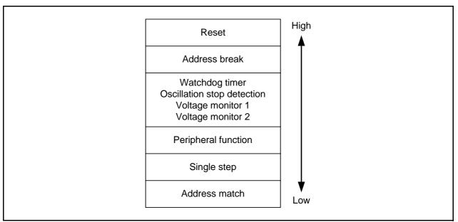
Figure 12.10 Priority Levels of Hardware Interrupts
