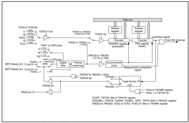
Figure 14.1 Block Diagram of Timer RA
