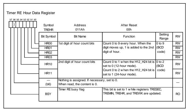
Figure 14.116 TREHR Register in Real-Time Clock Mode
