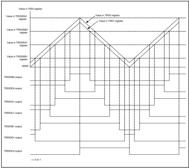
**Figure 14.95 Output Model of Complementary PWM Mode**
