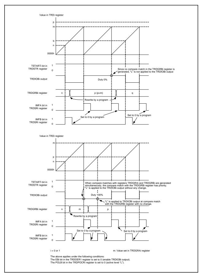
Figure 14.74 Operating Example of PWM Mode (Duty 0%, Duty 100%)
