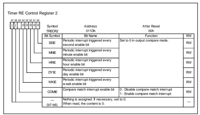
Figure 14.127 TRECR2 Register in Output Compare Mode
