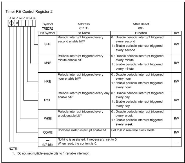
Figure 14.120 TRECR2 Register in Real-Time Clock Mode
