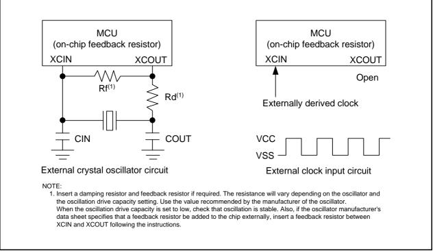
Figure 10.11 Examples of XCIN Clock Connection Circuits
