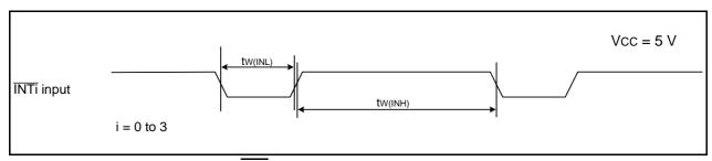
Figure 20.11 External Interrupt INTi Input Timing Diagram when Vcc = 5 V
