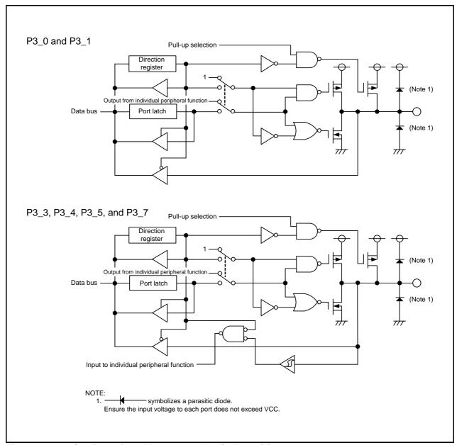
Configuration of Programmable I/O Ports (3) Figure 7.3
