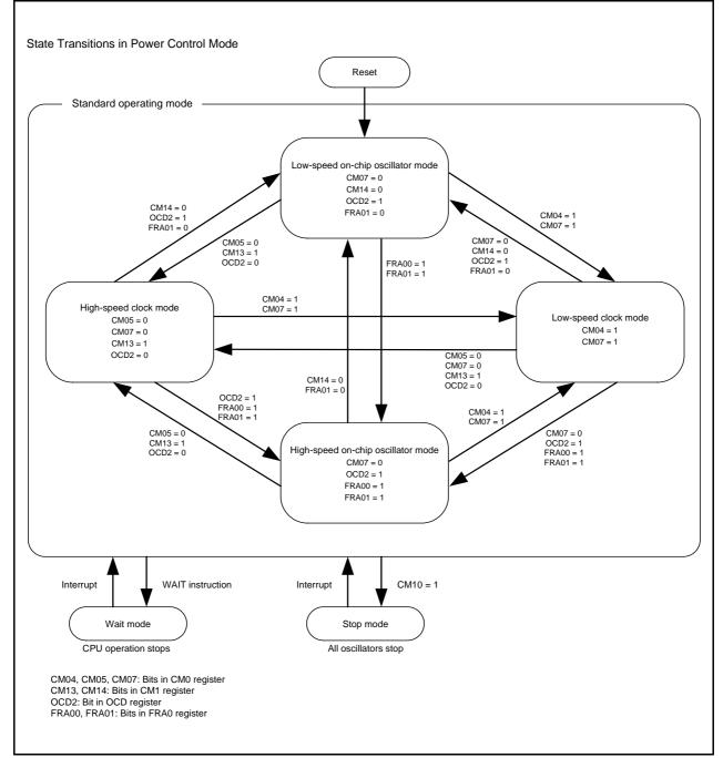
Figure 10.15 shows the State Transitions in Power Control Mode.
