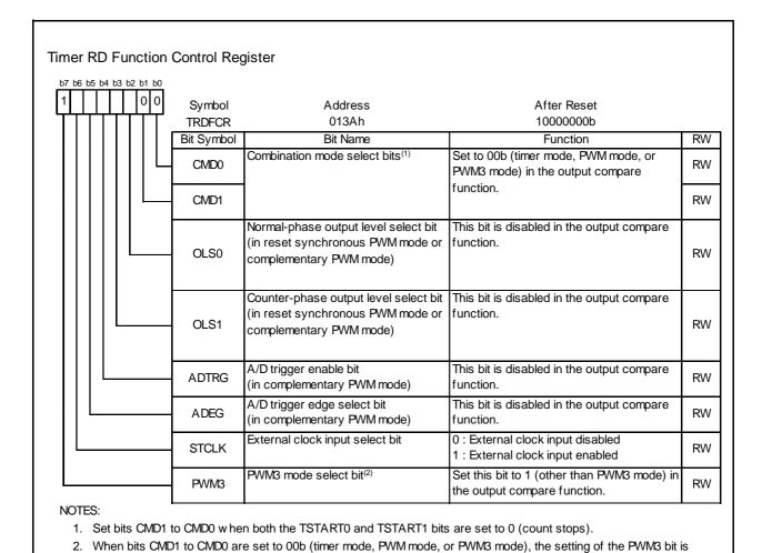
**Figure 14.49 TRDFCR Register in Output Compare Function**
