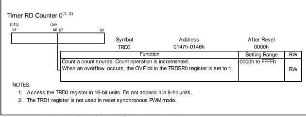
**Figure 14.82** TRD0 Registrar in Reset Synchronous PWM Mode
