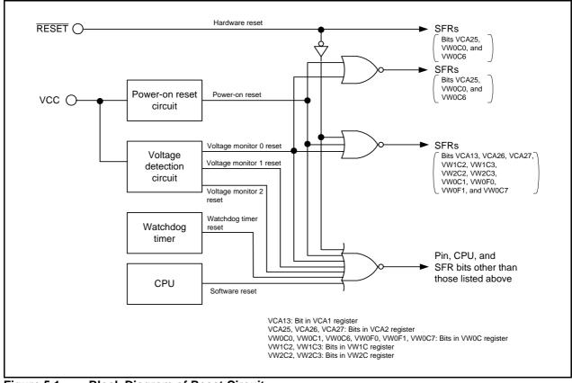
Figure 5.1 Block Diagram of Reset Circuit
