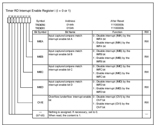
Registers TRDIER0 to TRDIER1 in Reset Synchronous PWM Mode **Figure 14.81**
