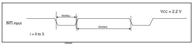
Figure 20.19 External Interrupt INTi Input Timing Diagram when Vcc = 2.2 V
