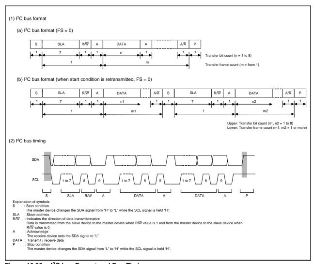
Figure 16.32 I<sup>2</sup>C bus Format and Bus Timing
