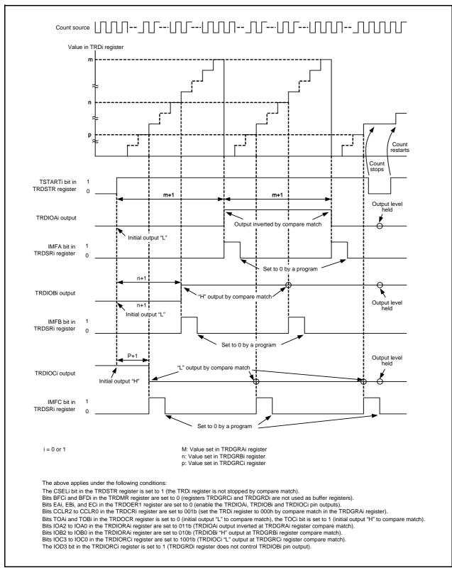
Figure 14.59 Operating Example of Output Compare Function
