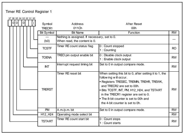
Figure 14.126 TRECR1 Register in Output Compare Mode
