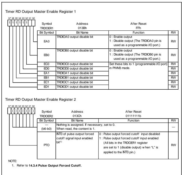
Figure 14.100 Registers TRDOER1 to TRDOER2 in PWM3 Mode
