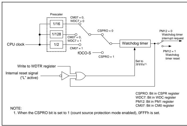
Figure 13.1 Block Diagram of Watchdog Timer
