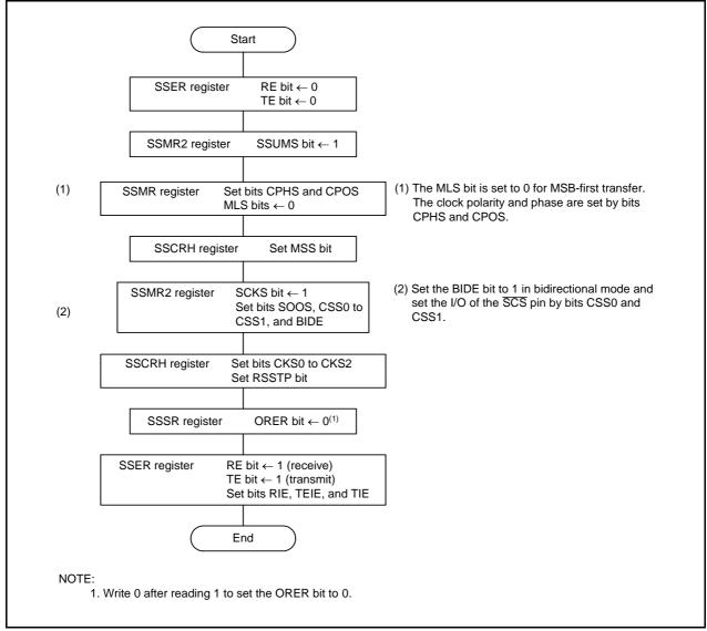
Figure 16.18 Initialization in 4-Wire Bus Communication Mode
