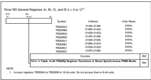
**Figure 14.83** Registers TRDGRAi, TRDGRBi, TRDGRCi, and TRDGRDi in Reset Synchronous PWM Mode
