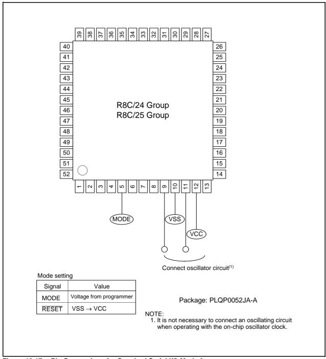
Figure 19.17 Pin Connections for Standard Serial I/O Mode 3
