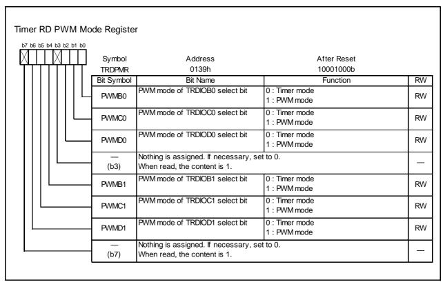
**Figure 14.64 TRDPMR Register in PWM Mode**
