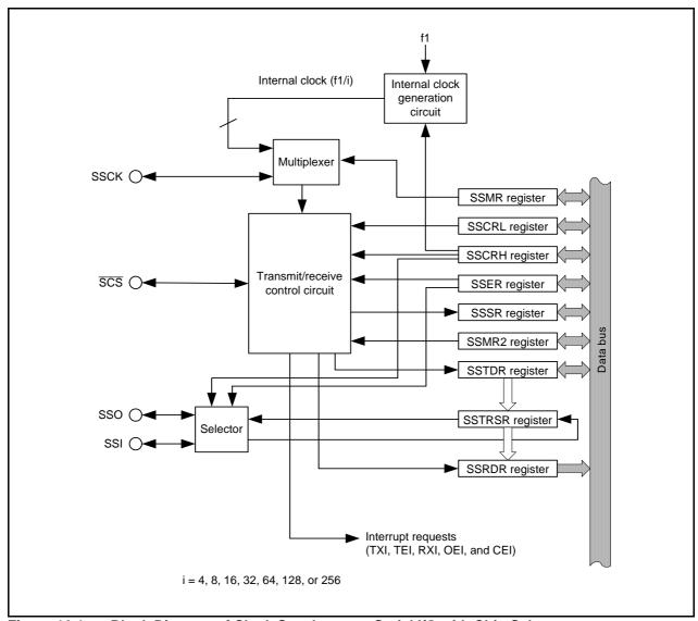
Block Diagram of Clock Synchronous Serial I/O with Chip Select Figure 16.1
