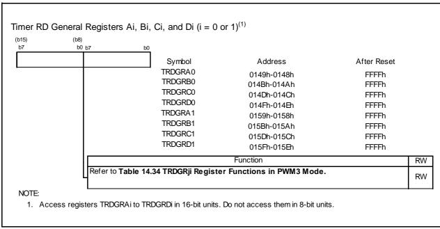
Figure 14.106 Registers TRDGRAi, TRDGRBi, TRDGRCi, and TRDGRDi in PWM3 Mode
