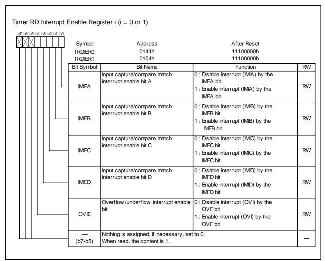
**Figure 14.69** Registers TRDIER0 to TRDIER1 in PWM Mode
