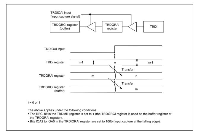
Figure 14.28 Buffer Operation in Input Capture Function
