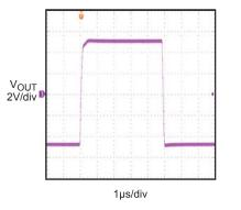
**Rail to Rail Output Response** V<sub>s+</sub>=+1.2V, V<sub>s</sub>=-1.2V, V<sub>IN</sub>=±0.22V, A<sub>V</sub>=-5
