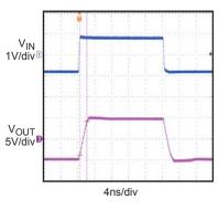
Large Signal Pulse Response V<sub>IN</sub>=±3V, A<sub>V</sub>=+1
