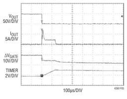
Figure 3. Short-Circuit Waveforms
