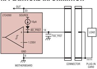
Figure 4. Plug-In Card Insertion/Removal
