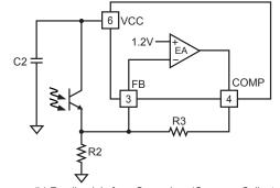
(b) Feedback is from Secondary (Common Collector)
