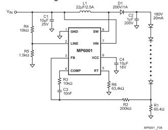
Figure 8—High Voltage LED Boost Controller Circuit
