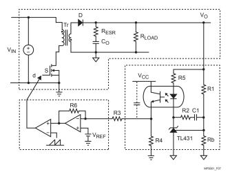
Figure 7—Simplified Circuit of Isolated Power Supply with Optocoupler Feedback The MP6001 uses current mode control to achieve easy compensation and fast transient response. A type II compensation network which has two poles and one zero is needed to stabilize the system. The practical compensation parameters are provided in the EV6001DN datasheet.
