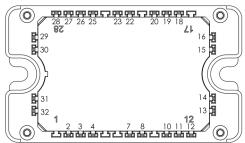
All multiple inputs and outputs must be shorted together; Example: 10/11/12; 7/8 ...
