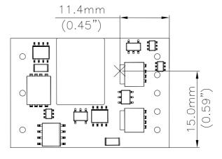
**Figure 21:** Temperature measurement location
