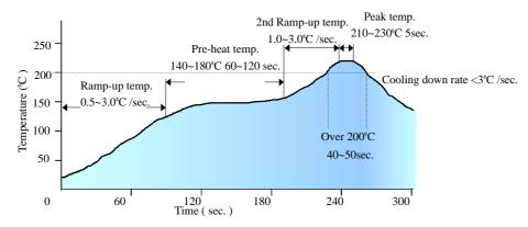
Note: The temperature refers to the pin of V48SR, measured on the pin +Vout joint.
