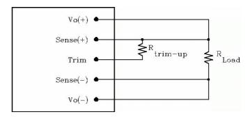
Figure 19: Circuit configuration for trim-up (increase output voltage)
