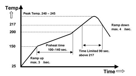
Note: The temperature refers to the pin of V48SR, measured on the pin +Vout joint.
