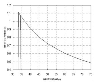
**Figure 3:** Typical full load input characteristics at room temperature Typical input characteristics at room temperature (lo=25A)
