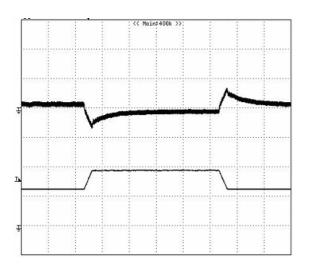
**Figure 8:** Output voltage response to step-change in load current (75%-50%-75% of lo, max; di/dt = 0.1A/μs). Load cap: 10μF tantalum capacitor and 1μF ceramic capacitor. Top Trace: Vout (50mV/div, 200us/div), Bottom Trace: lout (10A/div). Scope measurement should be made using a BNC cable (length shorter than 20 inches). Position the load between 51 mm to 76 mm (2 inches to 3 inches) from the module
