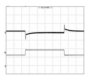
Figure 9: Output voltage response to step-change in load current (75%-50%-75% of lo, max; di/dt = 1.0A/µs). Load cap: 100µF tantalum capacitor and 1µF ceramic capacitor. Top Trace: Vout (50mV/div, 200us/div), Bottom Trace: lout (10A/div). Scope measurement should be made using a BNC cable (length shorter than 20 inches). Position the load between 51 mm to 76 mm (2 inches to 3 inches) from the module
