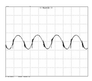
**Figure 11:** Input Terminal Ripple Current, i<sub>c</sub>, at full rated output current and nominal input voltage with 12µH source impedance and 33µF electrolytic capacitor (200 mA/div, 1us/div)
