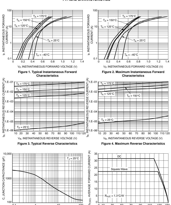
V<sub>R</sub>, REVERSE VOLTAGE (V) Figure 5. Typical Junction Capacitance
