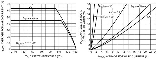
Figure 7. Current Derating per Device
