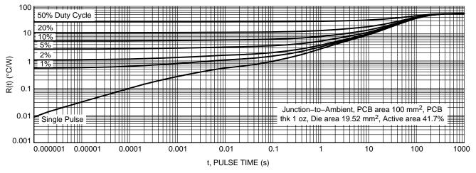
Figure 9. Thermal Characteristics
