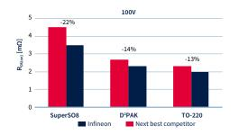
In the SuperSO8 package, OptiMOS™ 5 100V allows a two by one replacement of competitor parts enabling an even higher efficiency over the whole load range. This two by one replacement is without penalty in regard to thermal behavior. OptiMOS™ 5 100V has a 5V lower voltage overshoot compared to the next best competitor. In addition to isolated DC/DC as a primary application, the new OptiMOS™ 5 100V can also be utilized in Telecom application blocks including Or-ing, Hotswap and Battery Protection.
